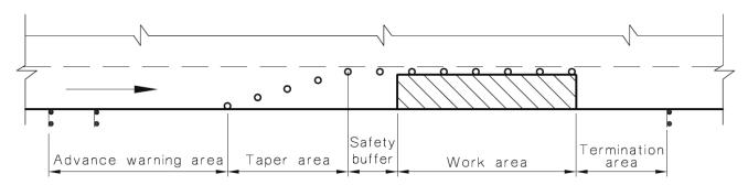
**Advance Warning Area:** The area before the work zone where signs and devices should be placed to warn road users that work is taking place and that there will be workers on or near the roadway.
